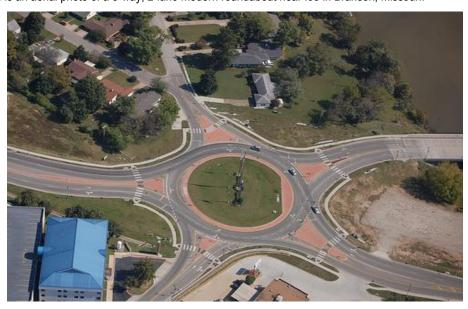
In the photo you can see the triangular medians at each street that deflect vehicles to slow traffic. Notice that the two entrances at the bottom of the photo are flared from one lane to two lanes to increase capacity. And, note
